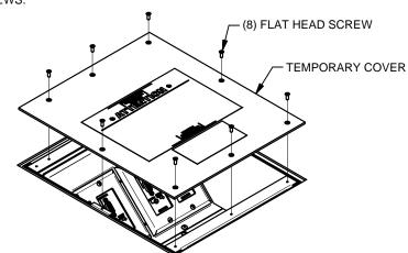
2. INSTALL CABLE INTERFACES AND CONNECTOR PLATES IF PREVIOUSLY NOT INSTALLED. CLEAN AREA IN AND AROUND ENTIRE TOP EDGE OF BOX AND APPLY 1/4" CONTINUOUS BEAD OF RTV SILICONE SEALANT.
