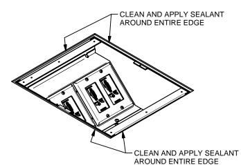
INSTALL SF8 ADAPTER PLATE (CAN BE ROTATED 180°) WITH SUPPLIED O-RINGS AND FLAT HEAD SCREWS. REFER TO SF8 COVER INSTALLATION INSTRUCTIONS TO COMPLETE INSTALLATION.
